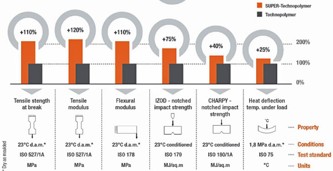
Comparison of Mechanical Properties between SUPER-Technopolymer and Technopolymer
